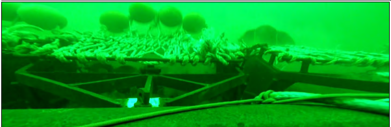
Figure 2. Limited Access General Category N-Viro modification trial frames. Top – Trial 1, bags with rubber chaffing gear and bags without rubber chaffing gear. Middle – Trial 2, frames with original N-Viro spring tines and frames with cutting bars replacing spring tines. Bottom – Trial 3, frames with float cans on bag and frames with kites on bag.
