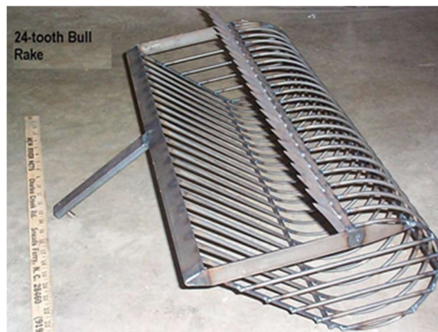
Figure 1. A typical bullrake used by commercial quahog harvesters in Rhode Island (Photo retrieved from https://www.newriversnets.com/nrn/shellfish.htm ).
