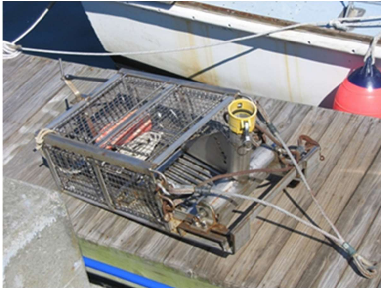
Figure 4. The hydraulic dredge utilized by RI DEM to assess quahog stocks in Narragansett Bay (Photo D. Leavitt).
