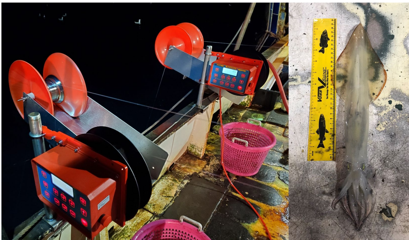
Two Belitronic BJ5000x jig machines set up to jig (left), and a long-finned squid caught by the jigs (right).
