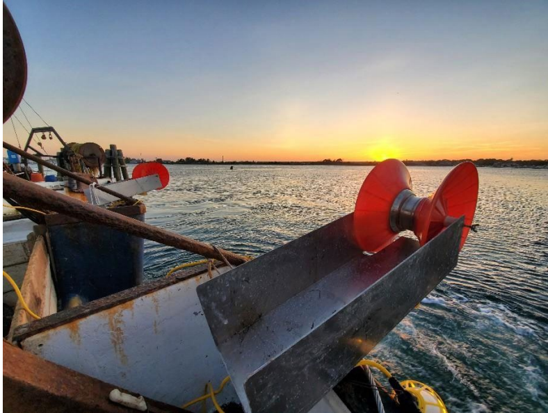
Figure 6: Two chutes and rollers mounted off the stern of the F/V Miss Edi with a string of construction lights hung below the chutes.
