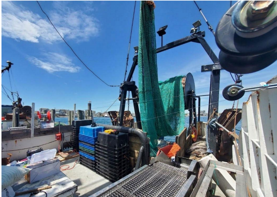
Figure 10: Cross deck image of the complete squid jigging setup on the F/V Hadley Ruth. Wheels on the right-hand side of the image are bolted through a similar wooden plank rail as seen on the left-hand side of the image.
