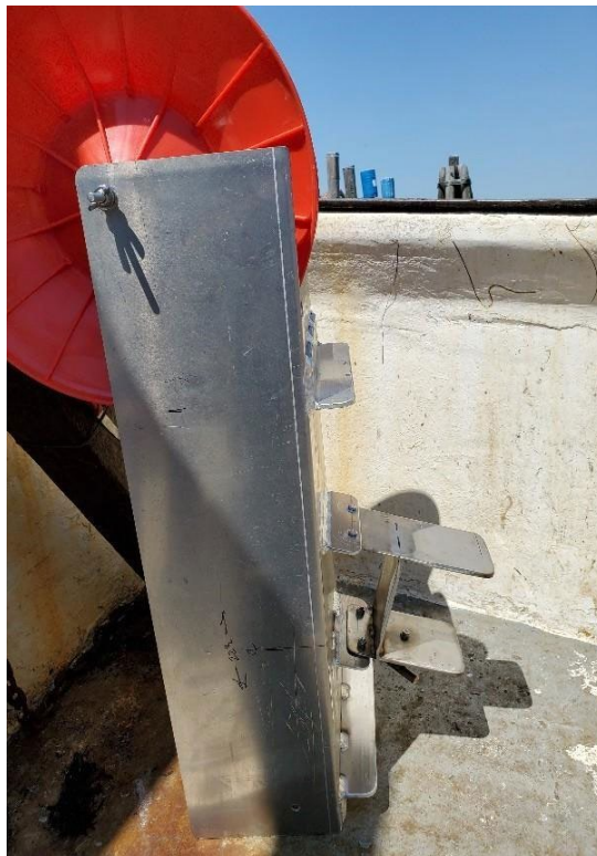
Figure 5: Fabricated brackets welded to the underside of each chute on the F/V Miss Edi. Each bracket slips over the rail and is held in place by tightening a threaded bolt.
