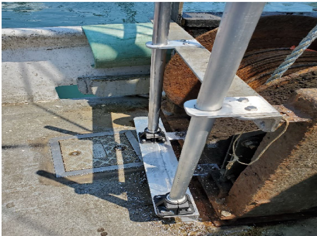
Figure 3: Jiggling machine mounting poles on the F/V Miss Edi. Mounting system is duplicated on both hydraulics on either side of the vessel so two machines could run simultaneously.
