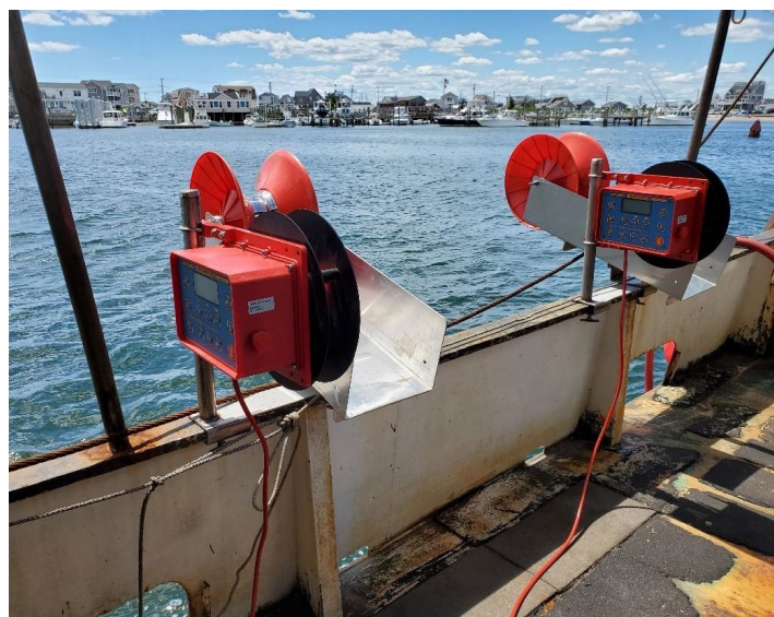
Figure 7: Squid jigging machines and chutes mounted as individual units on the starboard rail of the F/V Mattie and Maren.
