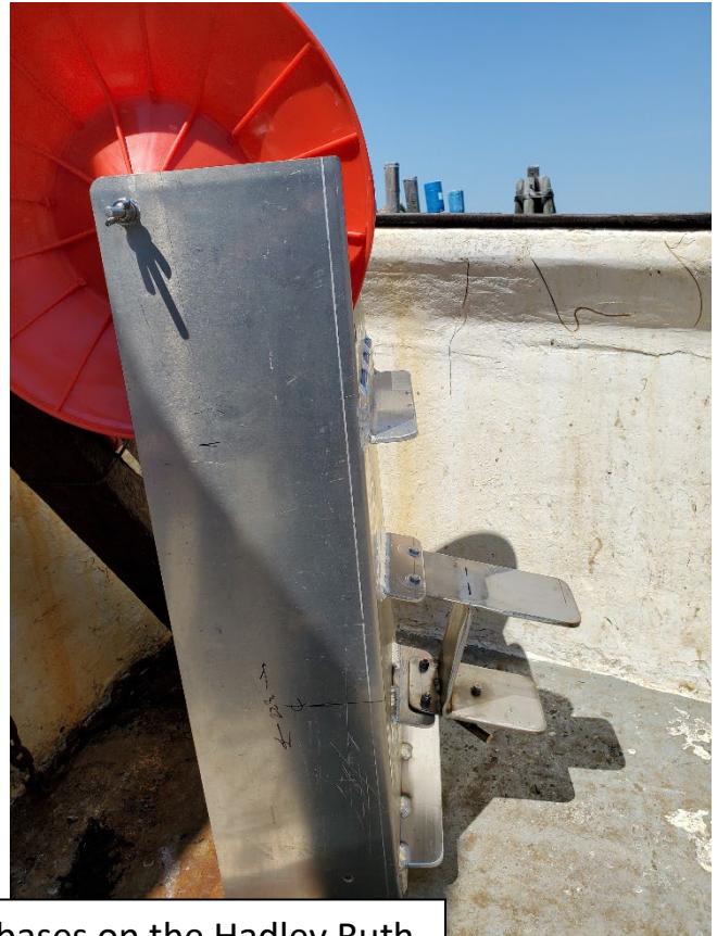
Support pole bases we drilled into the wooden bases on the Hadley Ruth
