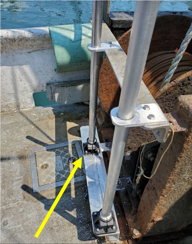
Support pole bases we drilled into the wooden bases on the Hadley Ruth
