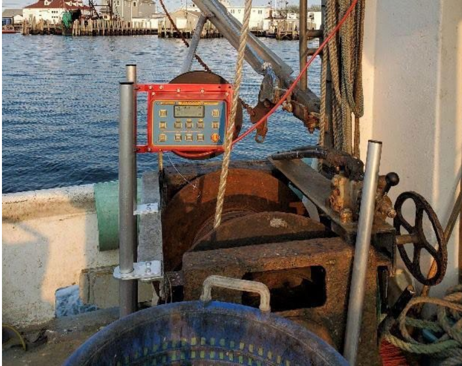
Figure 4: Jigging machine mounted on the support pole with line pulley above in the top right of the photo.
