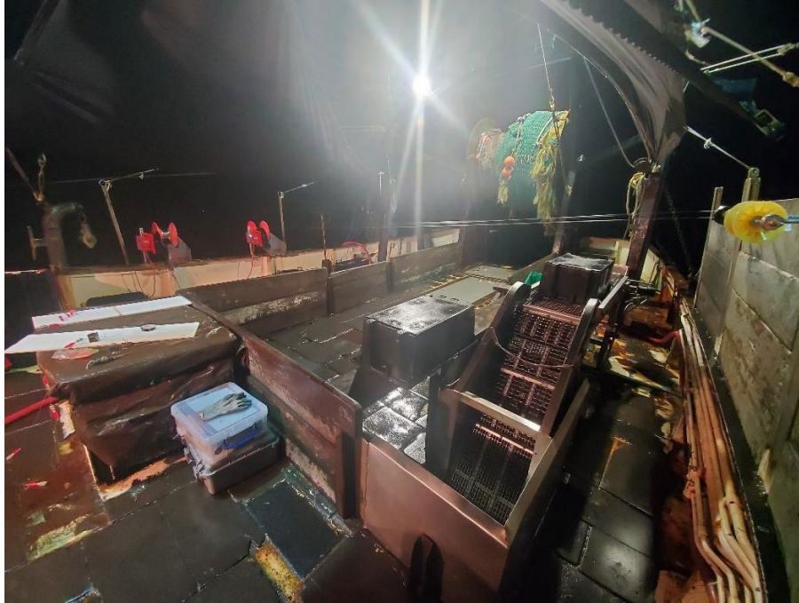
Figure 8: Two squid jigging machines installed on the F/V Mattie and Maren. The line travels from the reel on the machine to the portside of the vessel, through the rollers in the top right of the photo, and then overboard on the starboard side mounted chutes.
