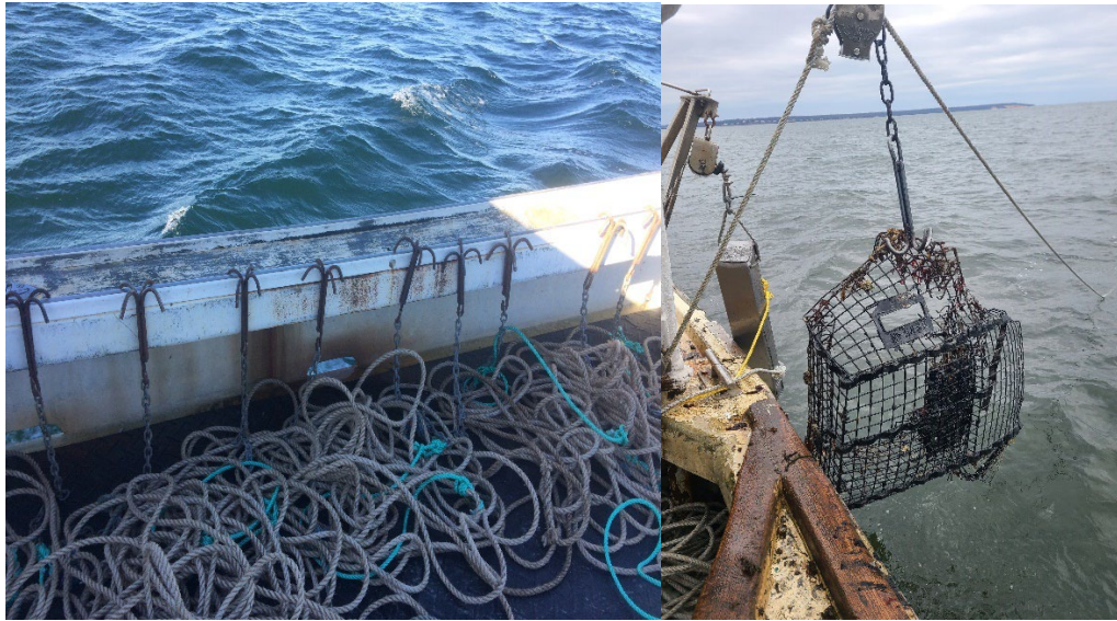
Figure 4. Example of specialized grapple equipment for removing ghost traps . Tor Vincent, Coastaldebrisgrappling Inc;
