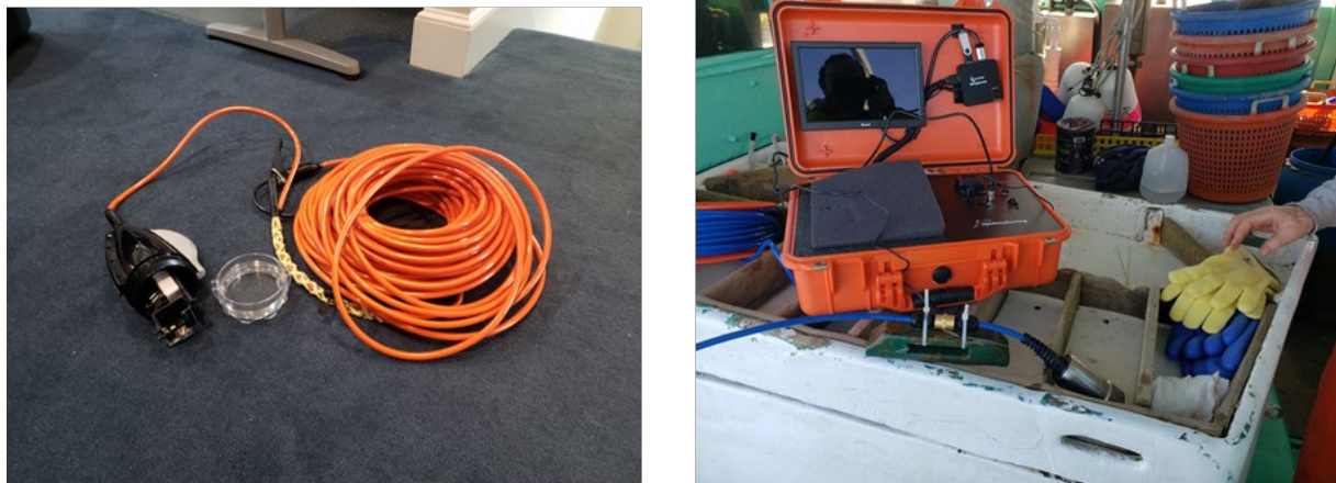
Figure 3. The Spot X (left) and Delta Vision (right) used for identifying ghost gear in Narragansett Bay, RI. The monitor (orange case) was used for both systems.
